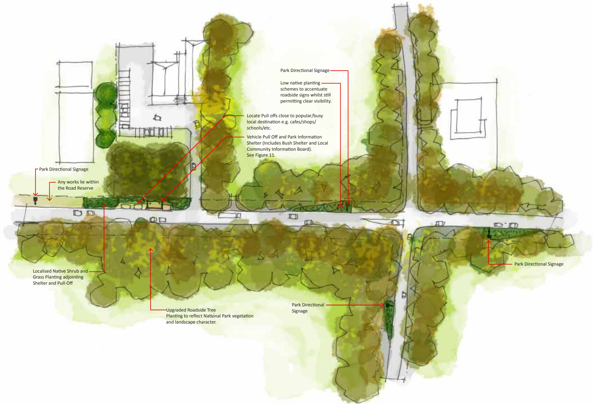
FIGURE 10. INDICATIVE DESIGN ELEMENTS - TYPICAL ROAD JUNCTION TREATMENTS
